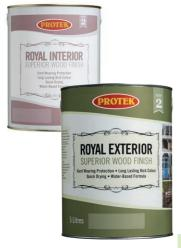
A 1 litre tin will cover approximately 8m² depending on moisture content and porosity of the timber. It is recommended that 2 - 3 coats be applied. Royal Exterior Wood Finish is a high build formulation so each extra coat increases the colour and sheen. No primer or basecoat required. If applying to bare timber a knotting agent or stain blocking primer should be applied prior to Royal to prevent any possible resin bleed staining the coating.
